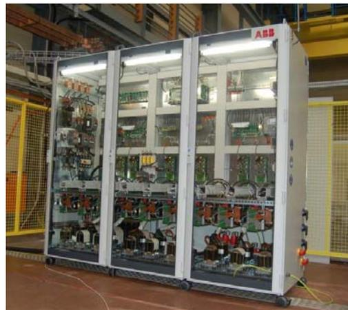
Fig. 10. ABB low voltage PET prototype (2011) [19].
