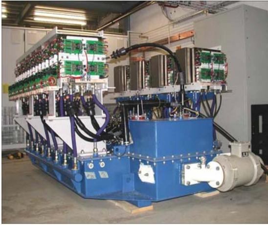
Fig. 5. ABB PET prototype (2006) using topology from Fig.4 [5].
