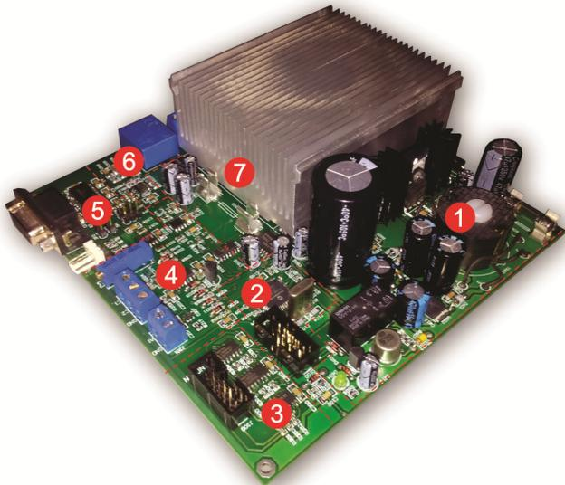
Fig. 1. AMD-HD DC motor drive.
