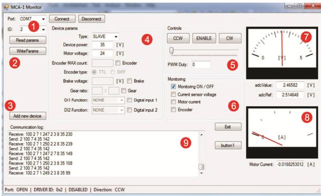
Fig. 2. Main window of MCA-1 monitor GUI
