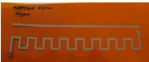
Fig. 8. Meander inductor on flexible Kapton substrate.
