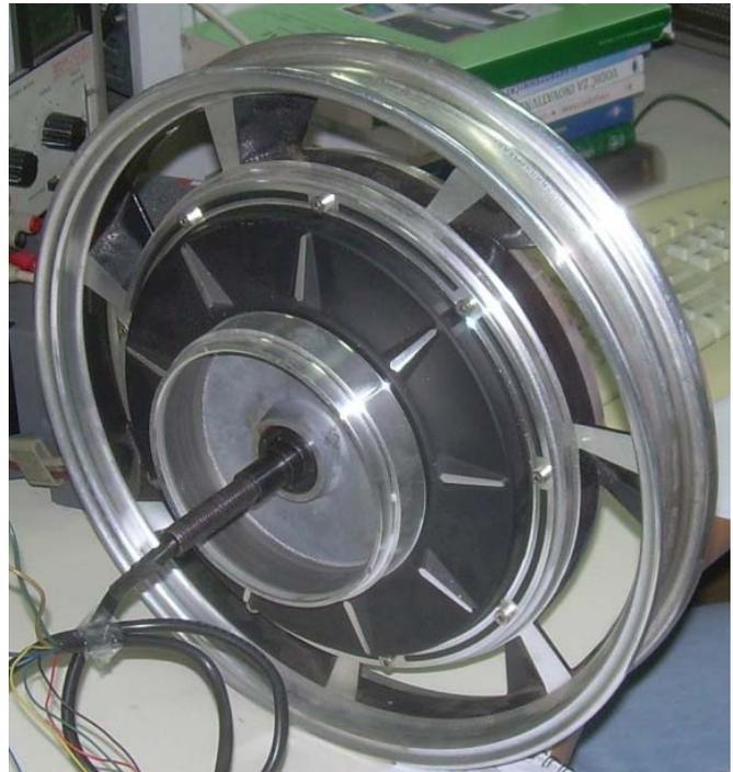
Fig. 1. The explored 300W outer rotor BLDC motor.
