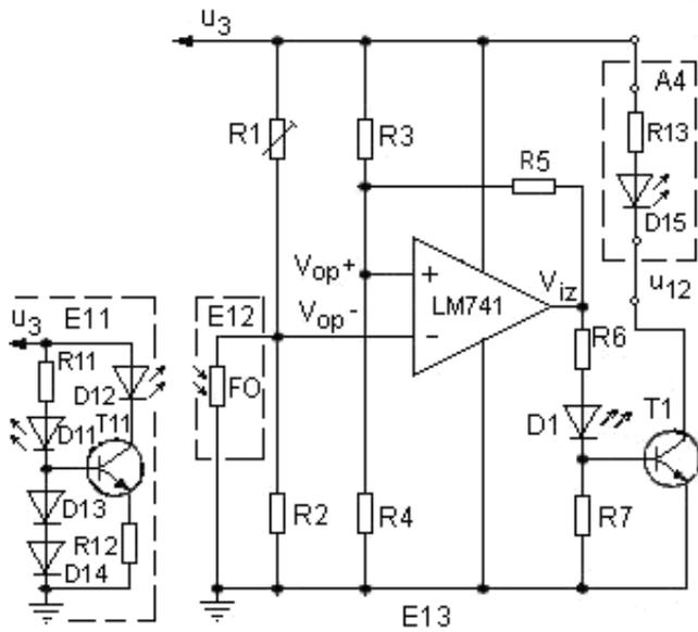
Fig. 6. Circuits of transmitter E11 and receiver E12/E13.
