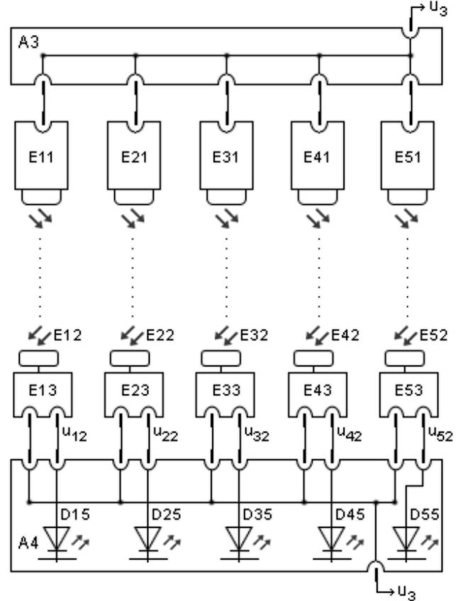
Fig. 5. Block scheme of system for determining coordinates.
