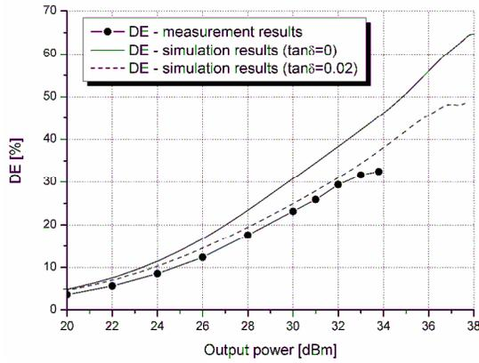
Fig. 8. Drain efficiency of two-way Doherty amplifier.
