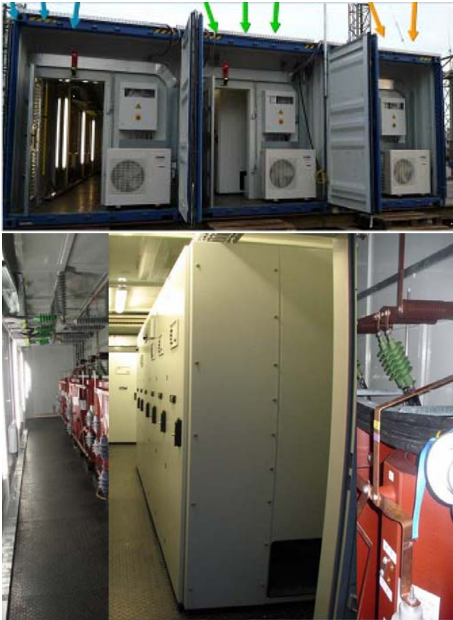
Fig. 9. Photographs of a sag generator.
