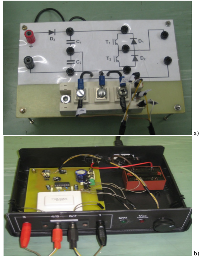
Fig. 5. Power section a) and control unit b) of inverter.
