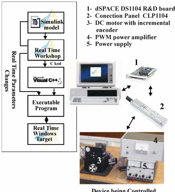
Fig. 4. Schematic representation of experimental setup.
