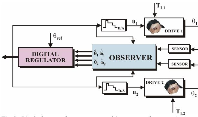
Fig. 2. Block diagram of a servo system with cross-coupling control.
