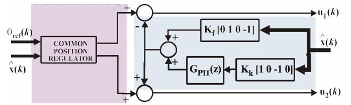
Fig. 3. Structure of digital regulator in the positioning servo system with cross-coupling control in Fig. 2.
