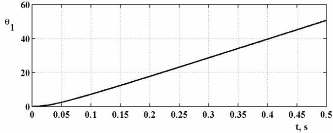
Fig. 5. Step response of servo drive angular position which is measured by using incremental encoder with 1000 pulses per revolution; input signal is  $u_1(t) = 10 \cdot h(t)$ .
