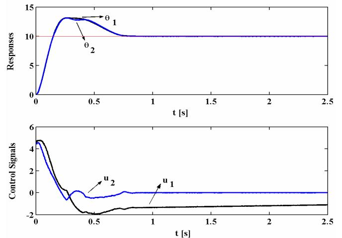
Fig. 8. Responses of angular positions and control signals of digital regulator after step reference signal.
