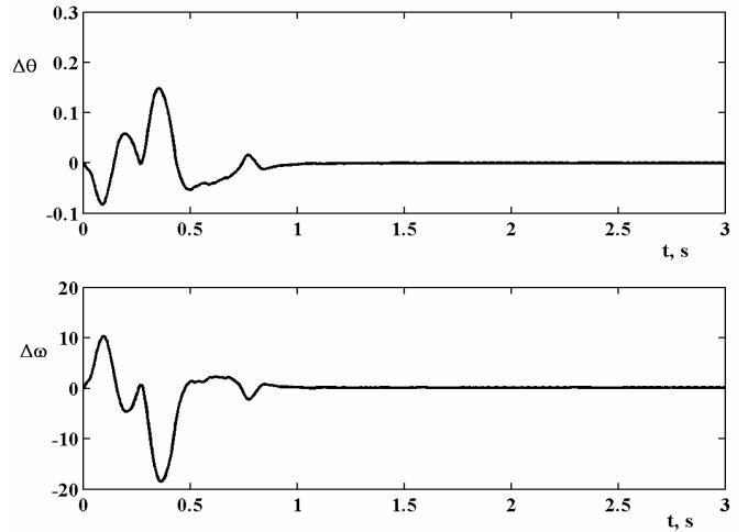
Fig. 7. Transient response and steady-state values of position and speed differences.
