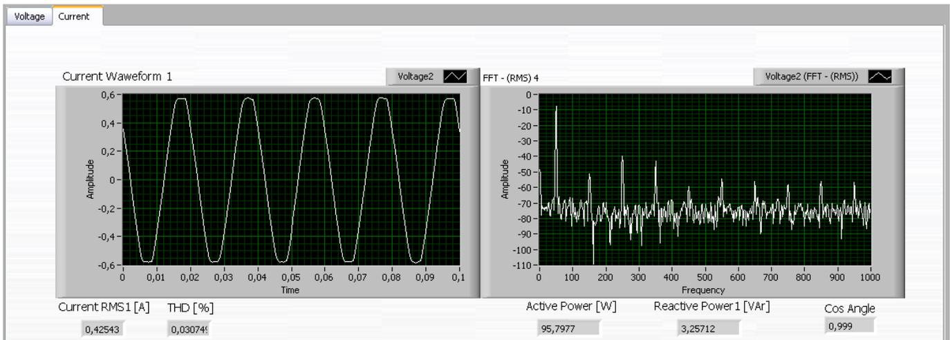
Fig. 6. Front panel of the virtual instrument for current and power measurements
