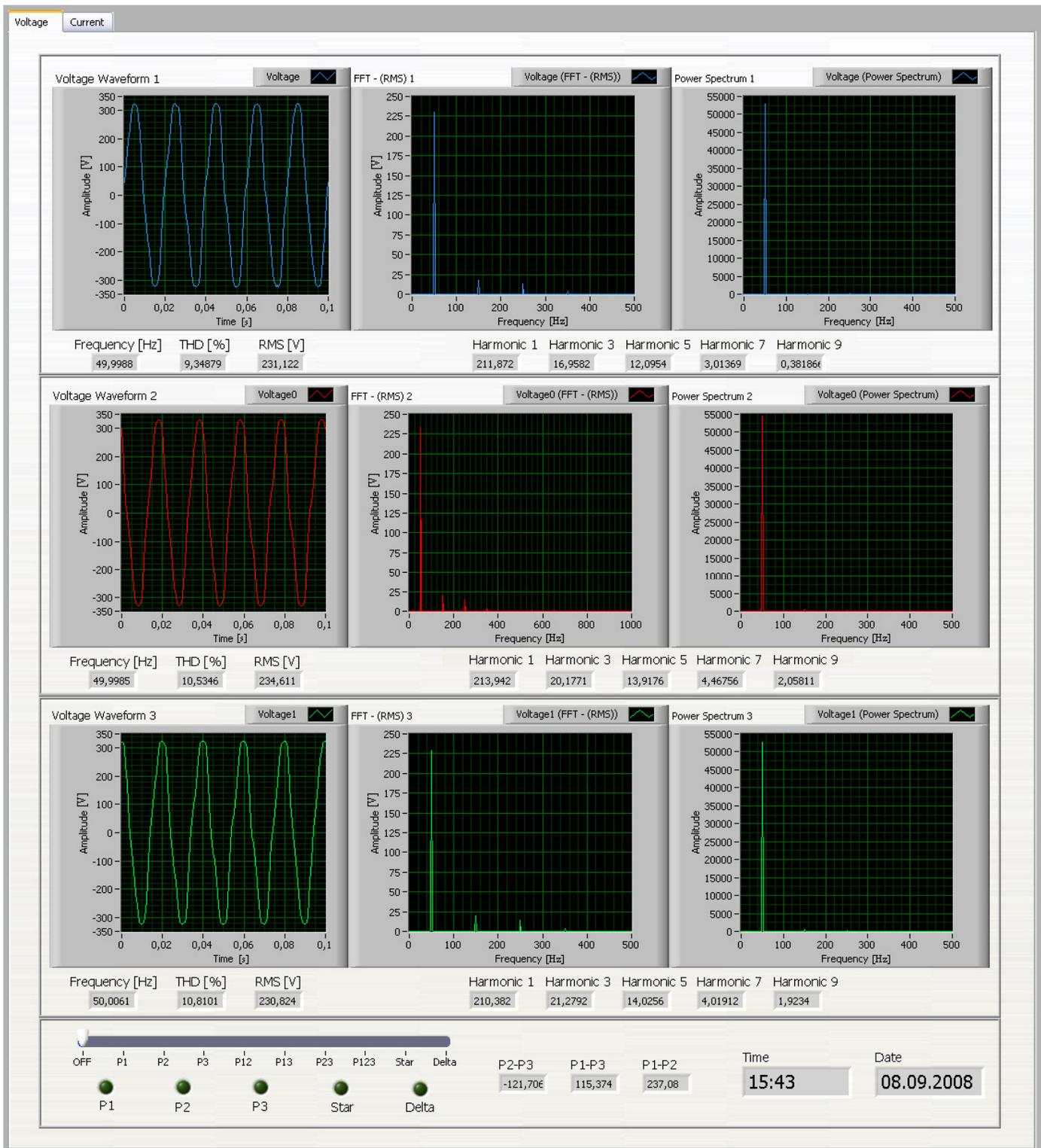
Fig. 4. Front panel of the virtual instrument
