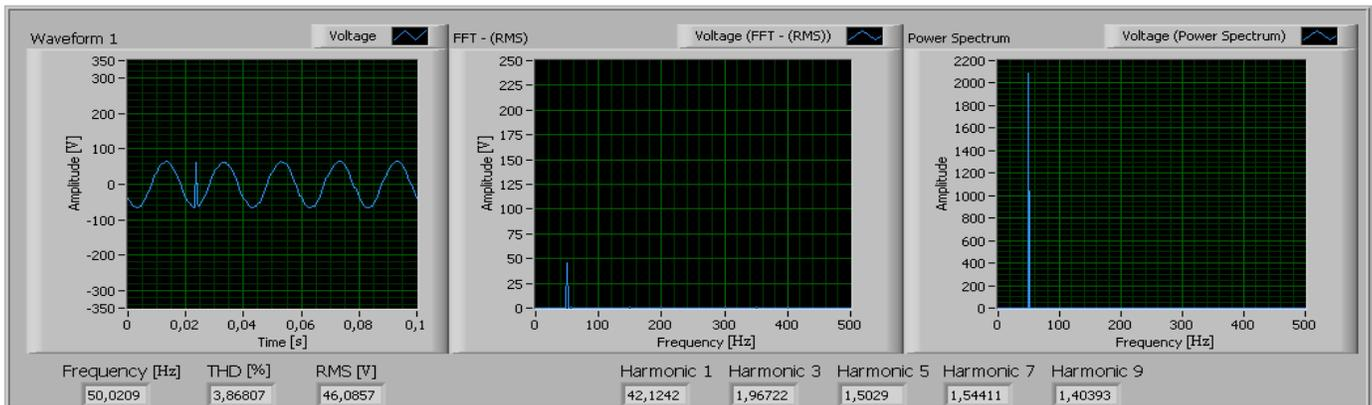
Fig. 8. High transient pulse caused by lightning
