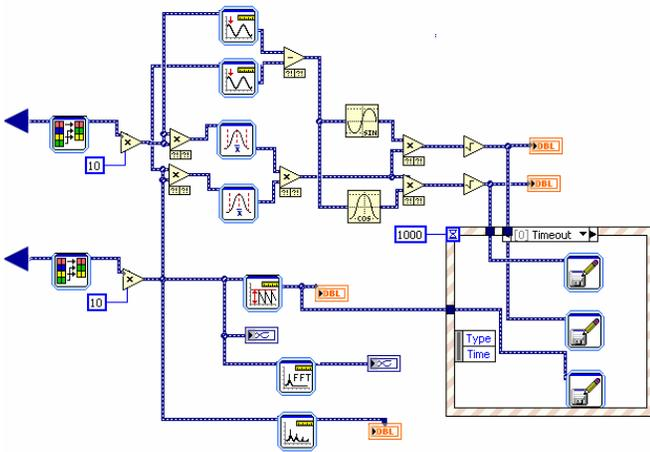
Fig. 5. Current and power measurements block diagram
