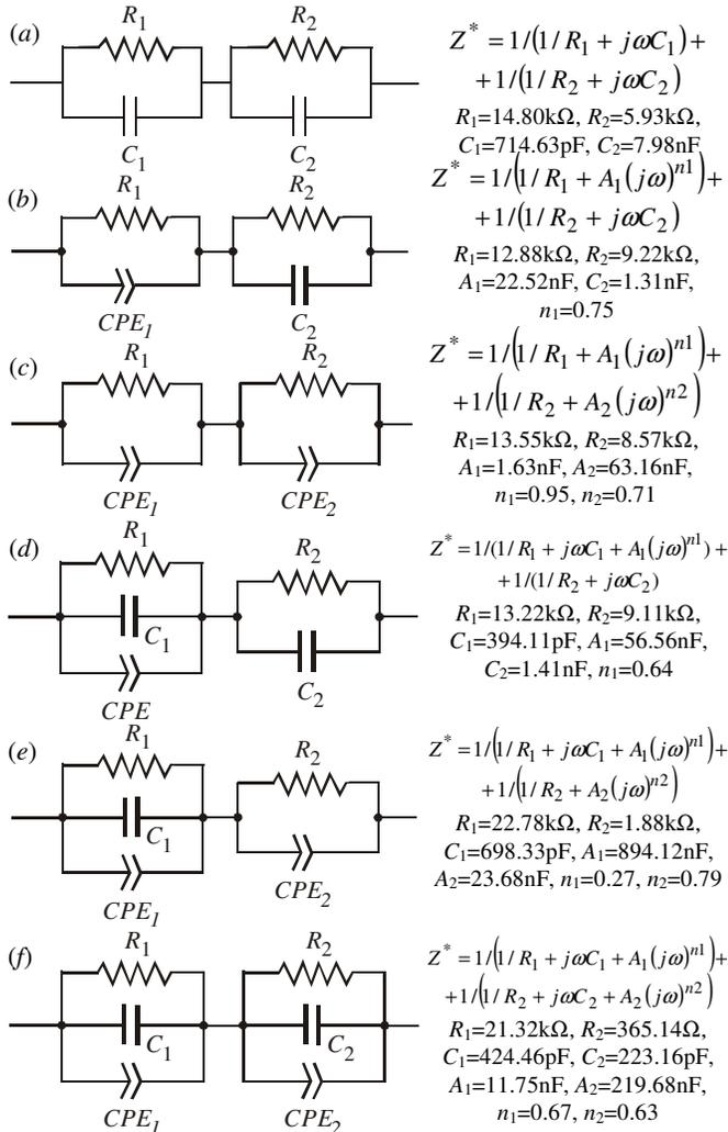
Fig. 12. Various equivalent circuits to model La-BT ceramic
