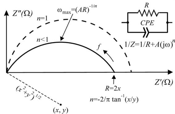
Fig. 11. Modelled complex impedance characteristic for equivalent R-CPE circuit, shown as inset in the image
