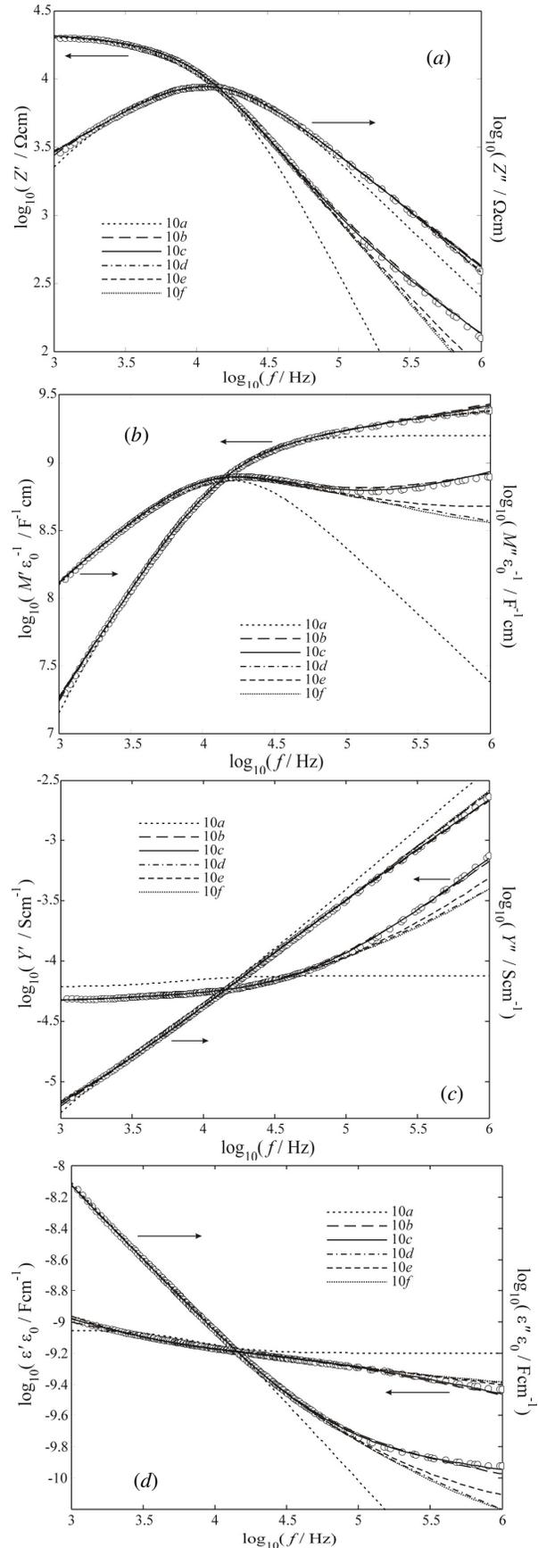
Fig. 13. Normalised frequency dependences of real and imaginary impedance parts for (a)  $Z^*$ , (b)  $M^*$ , (c)  $Y^*$  and (d)  $\epsilon^*$ , in log-log ratio, measured at  $350^\circ\text{C}$  (circles), and modeled results obtained through best fitting for equivalent circuits presented in figure 12 (colored lines)
