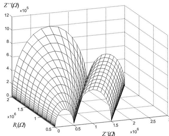
Fig. 3. Impedance of equivalent circuit from Fig.1 shown in complex plane  $Z''(Z')$ , where:  $C_1=10^{-12}$ F,  $C_2=10^{-9}$ F,  $R_2=10^6\Omega$ , and  $R_1$  changes in the range from  $0.5 \times 10^8\Omega$  do  $2 \times 10^6\Omega$
