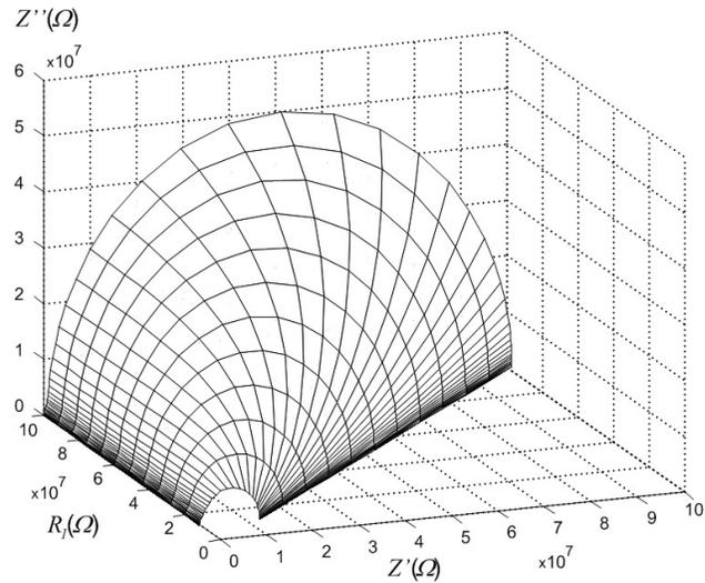
Fig. 2. Impedance of equivalent circuit from Fig.1 shown in complex plane  $Z''(Z')$ , where:  $C_1=C_2=10^{-12}$ F,  $R_2=10^6\Omega$ , and  $R_1$  changes in the range from  $5 \times 10^8\Omega$  to  $10^8\Omega$
