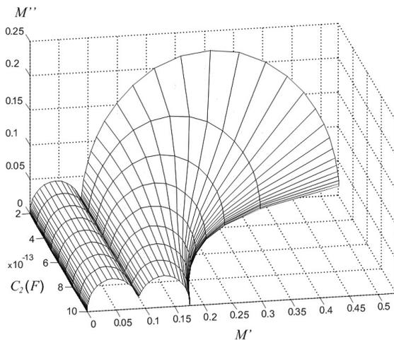
Fig. 5. Electrical modulus of equivalent circuit from figure 1 shown in complex plane  $M''(M')$ , where:  $R_1 = 10^8 \Omega$ ,  $R_2 = 10^6 \Omega$ ,  $C_1 = 10^{-12} \text{F}$ , and  $C_2$  changes over the range  $0.2 \times 10^{-12} \text{F}$  to  $10^{-12} \text{F}$
