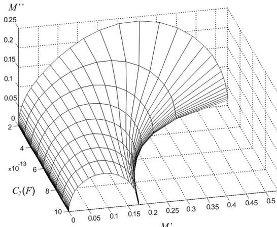
Fig. 4. Electrical modulus of equivalent circuit from figure 1 shown in complex plane  $M''(M')$ , where:  $R_1 = R_2 = 10^6 \Omega$ ,  $C_1 = 10^{-12} \text{F}$ , and  $C_2$  changes in the range from  $0.2 \times 10^{-12} \text{F}$  to  $10^{-12} \text{F}$
