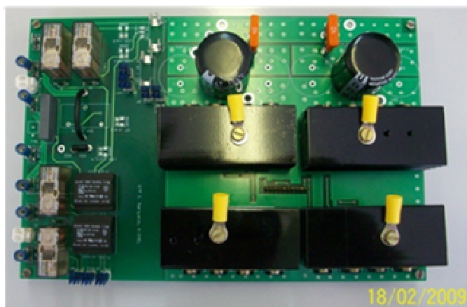
Fig. 9. Compact inverter power stage on PCB.
