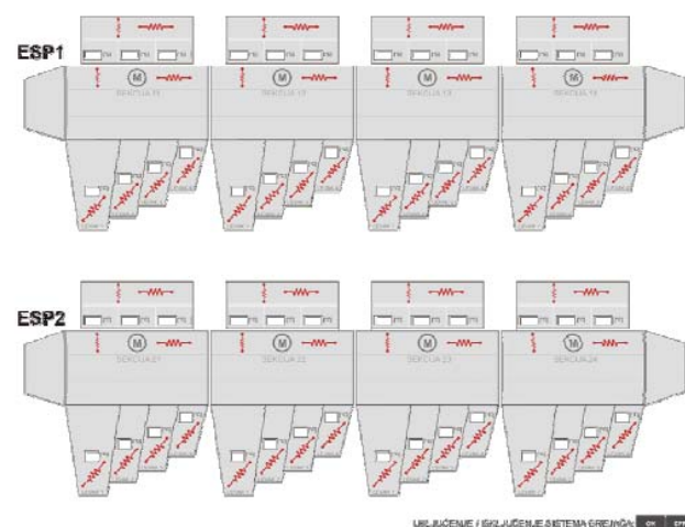
Fig. 16. Front panel view of the PLC functions related to the ceramic insulator pre-heating.
