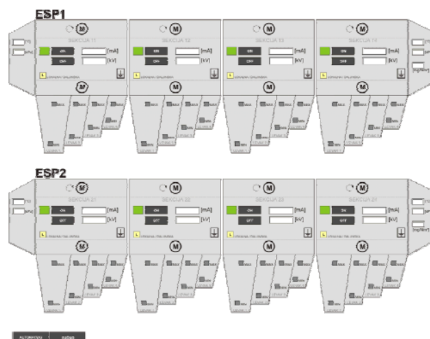
Fig. 15. Front panel view of the PLC functions related to the ESP rapping control.
